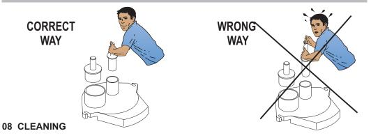
IMPORTANT BEFORE to clean the machine unplug it from the electric network . Always be sure that the Disc is completely still.
