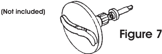
Shredding assembly, with 5/16 Shredder Plate.
