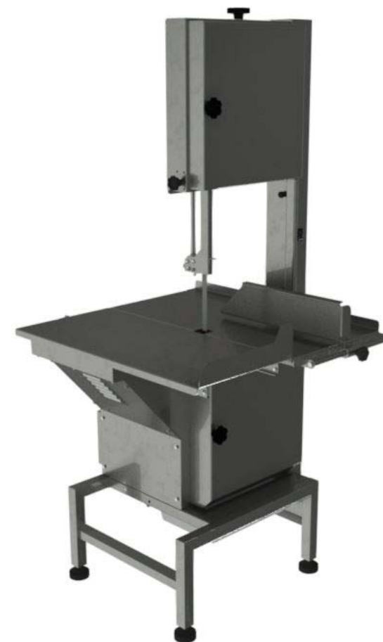
BAND SAW STAINLESS STEEL, MOVABLE TABLE, THICKNESS GUIDE, BLADE 3.150 mm
