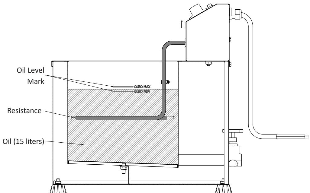
Oil levels are shown in FIGURE 03, for a perfect operation and enhanced safety it is necessary a strict respect for the oil levels.
